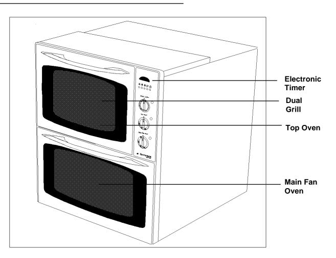
Your built in appliance comprises of a conventional oven and dual grill in the top compartment. The top oven is convenient and economical for mid-week use because of its size.
